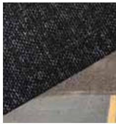
These heavier weight fabrics are designed for applications where higher strength, stability and performance is necessary. This fabric is one of the most commonly used geotextiles for road stabilization, ground stabilization and aggregate separation. Made of polypropylene, the geotextile is UV resistance as well as being resistant to commonly encountered soil chemicals, mildew and insects. Non-biodegradable. Polypropylene is stable within a pH range of 2 to 13, making it one
